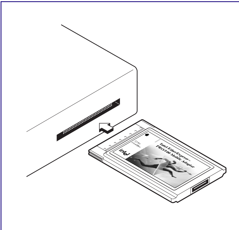
Inserting the PRO/100 CardBus adapter into the Computer
